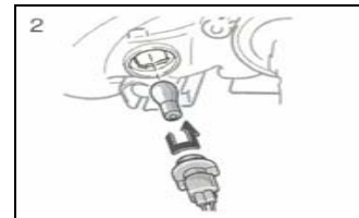
2. Turn the bulb clockwise and pull it out, and then remove it.
